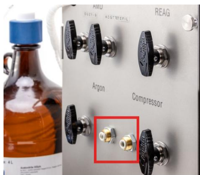
Figure 4-3: Gas line connections
