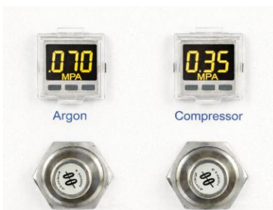
Figure 5-1: Verify compressor pressure readings
