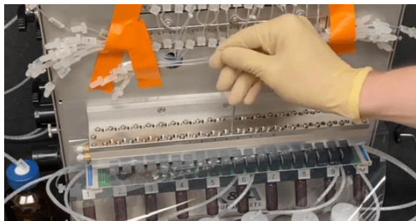
Figure 6-3: Inspecting luer fittings under columns
