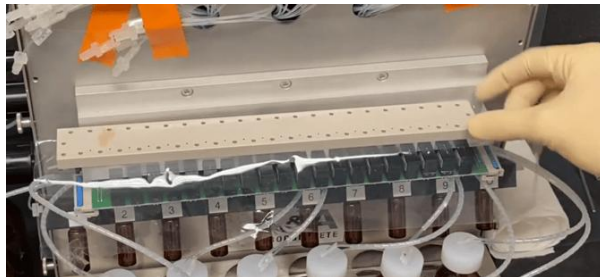
Figure 6-2: Aligning new membrane — channels facing downward
